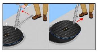
**ONLY use the MwayPro Lifting Tool!** Evidence of using any other device may damage the product & invalidate warranty
