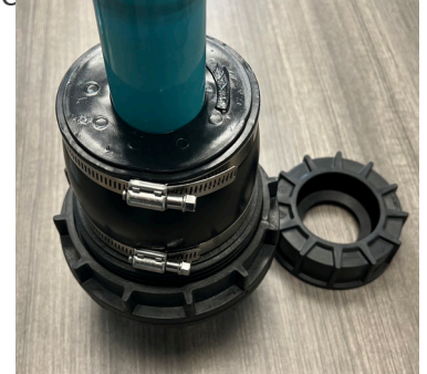
Example of APT Repaired
